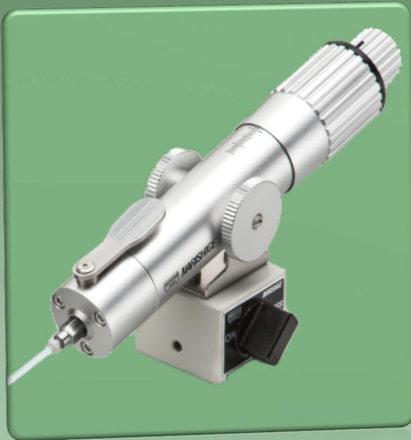
When the pressure relief valve is pressed, the syringe inside the injector becomes balanced immediately at one atmospheric pressure (1 atm.)
